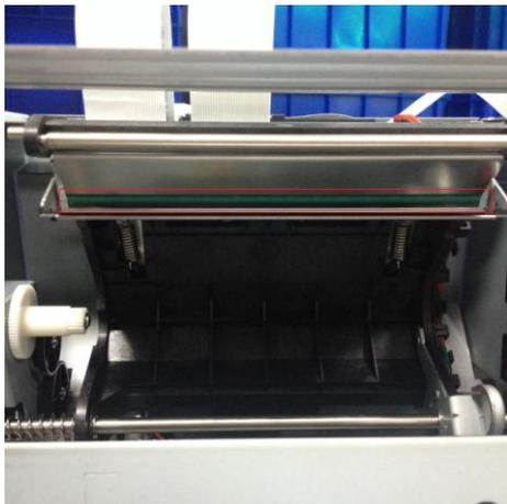
6.1 Use Gauze: Clean the heating element (glass bar) of the Thermal Printing Head with ethyl alcohol
