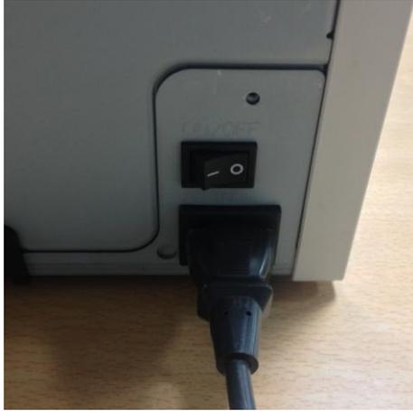
4.1 Connect the printer power cord to the AC IN slot
