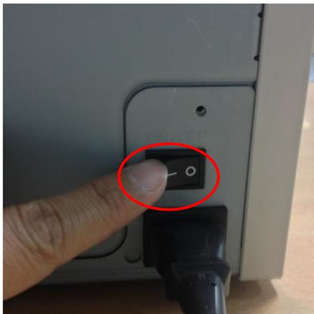
4.3 Powering up the printer. As printing is in running, do not power off the printer.
