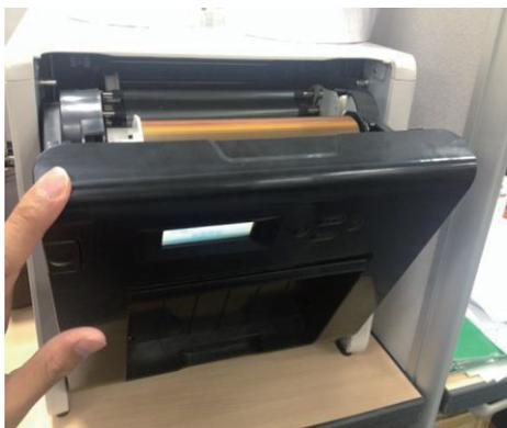
4.7 Closing front cover and 4 sheets of paper will be cut without printing automatically to ensure the paper quality.
