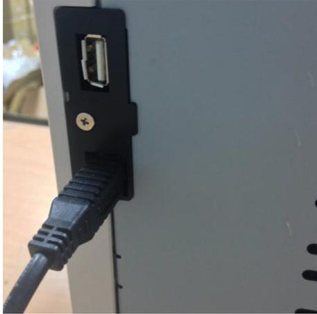
4.2 Use USB cable to connect printer and PC
